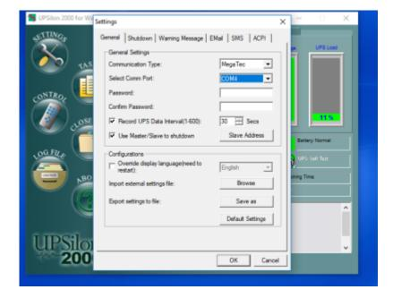
If these steps have been done correctly the software package should indicate that the UPS is connected to the PC as shown in the image below. One thing to try if it is not detecting is to restart the software Package.
