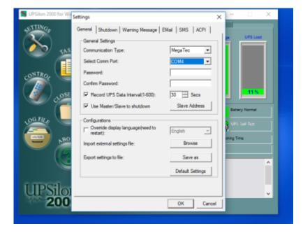
If these steps have been done correctly the software package should indicate that the UPS is connected to the PC as shown in the image below. One thing to try if it is not detecting is to restart the software Package.
