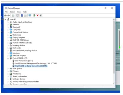
Once you have established what COM port your UPS is plugged into select that port on the included software as shown in the image below (out USB to Serial adaptor is now on COM4)
